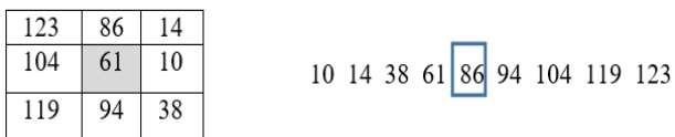
Figure. 1 Illustration of calculating the value in an image with a kernel size of 3x3
