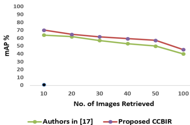
Figure 9 Mean Average Precision Score Comparison with varying number of retrieved images for Corel-10K
