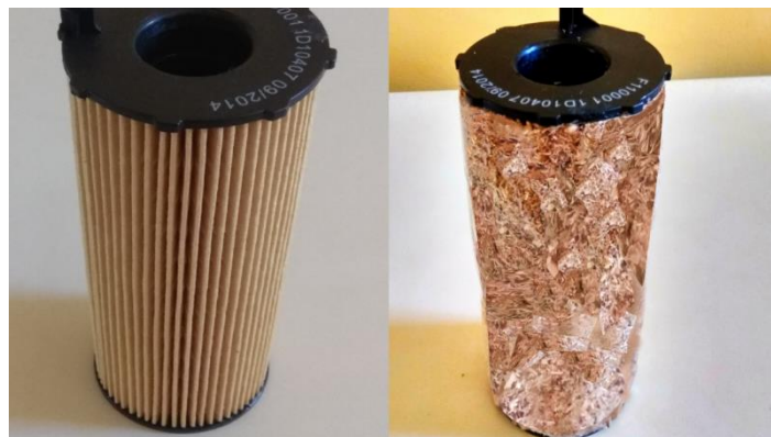
Fig. 1. OEM and modified engine oil filter comparison
