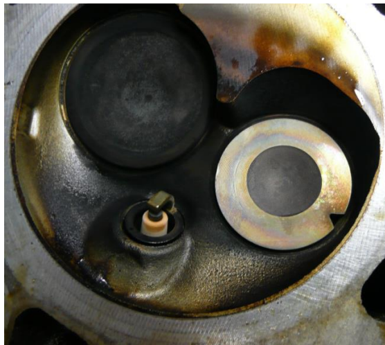
Fig. 2. Modeled damage to the spark ignition engine exhaust valve
