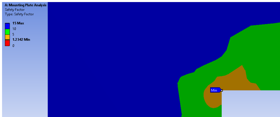
Fig. 5. Mounting plate FEA safety factor (close-up)
