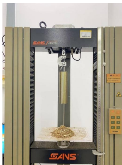
Fig. 1 – Physical test of angle of repose by cylinder lifting method
