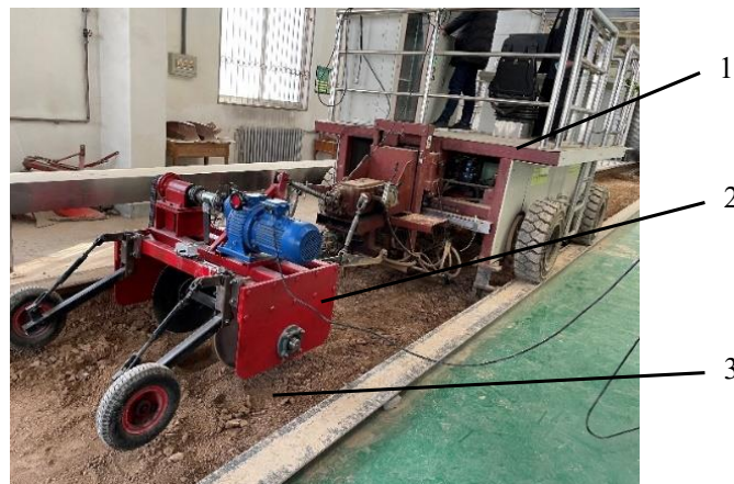
a. Hitch on the testing vehicle of soil bin 1. Testing vehicle 2. Designed test bench 3. Soil bin
