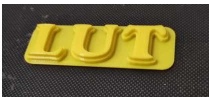
Fig. 2. Printed 3D model with dimensions: 6.0 mm × 3.6 mm × 3.5 mm. LUT – Lublin University of Technology
