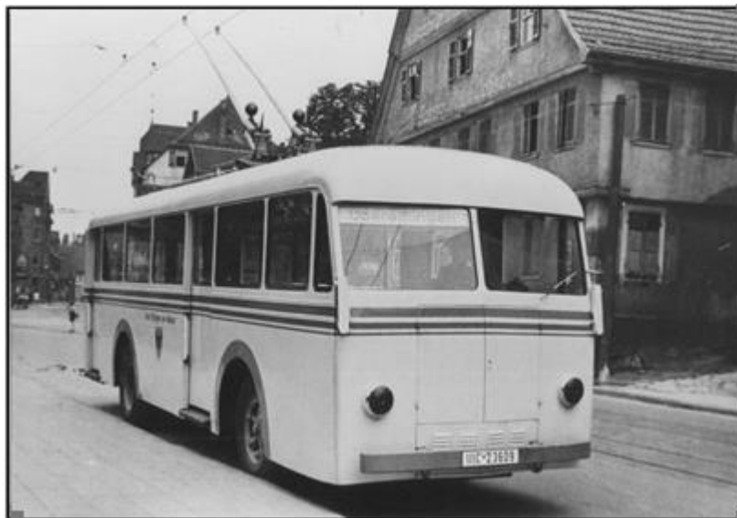
Figure 6. MAN MPE 4500 I/Kassbohrer/BBC trolleybus produced in 1944 with standard current collectors and camouflaged headlights in Esslingen (pictured late model on MAN MPE I chassis) (Kiebler, Ronald, 2000b).
