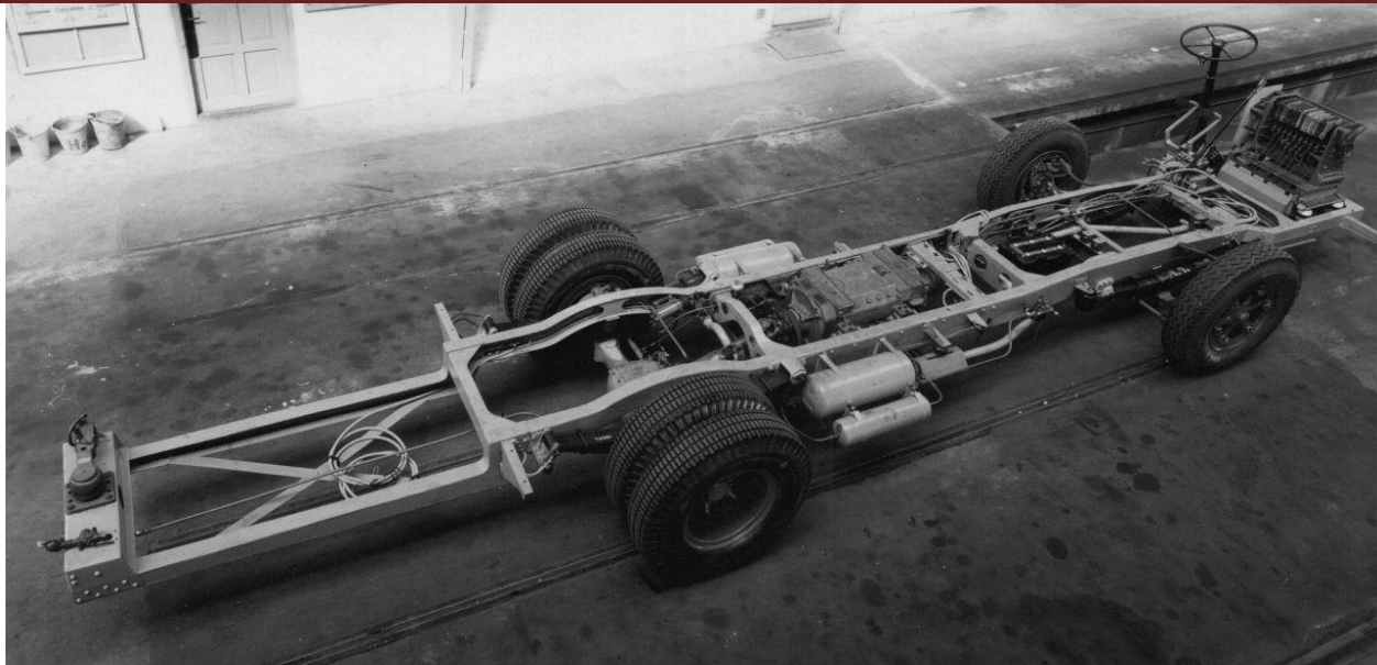
Figure 1. MAN MPE I standard trolleybus chassis, the 1940s model. The wheelbase is 4.25m, which is 1m less than in the early cars of the 1938 model. Also, early trolleybuses (Chernivtsi, Zwickau) had a rear axle single-tire wheel (in the photo – a classic double-tire wheel) (Kiebler, Ronald, 2000a).
