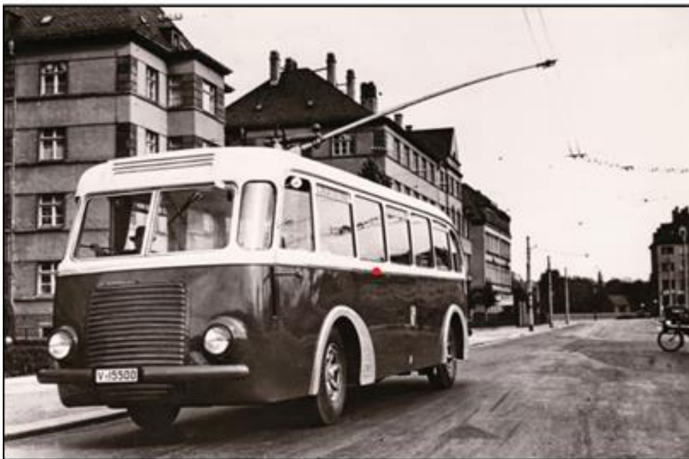
Figure 4. MAN MPE I/Schumann/BBC trolleybus produced in 1938 with a single-rod current collector in Zwickau (the two-pole rod was later replaced by two conventional collectors) (Gorodskoj elektrotransport, 2002–2021a).
