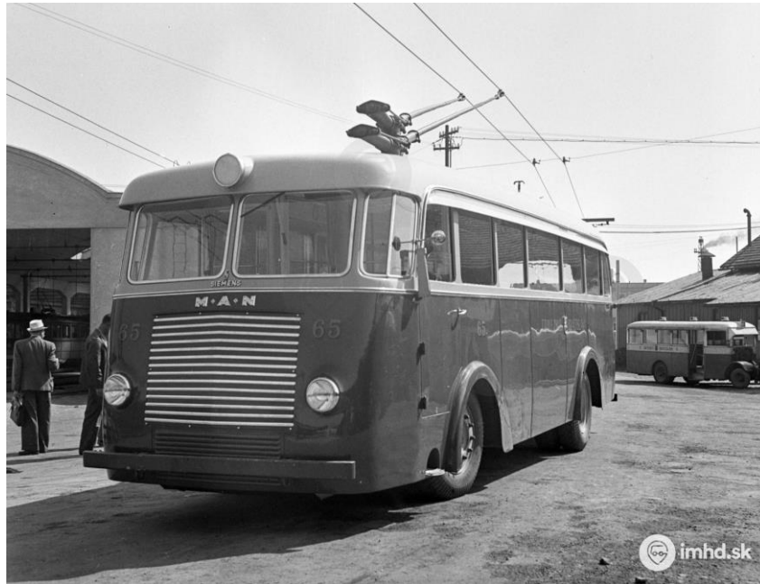
Figure 5. MAN MPE 4500 I/Sodomka/SSW trolleybus produced in 1940 with current collectors mounted on one axle in Bratislava (then Czechoslovakia) (Popis typu vozidla..., n. d.).
