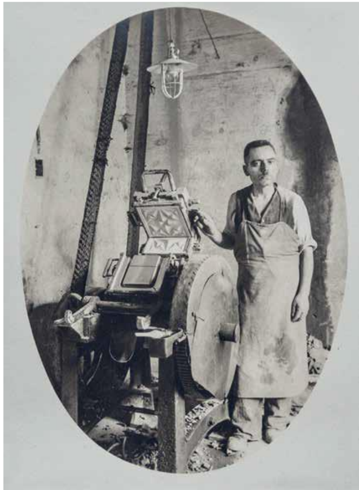
Figure 5. Press for the manufacture of tiles at the factory of I. Levynsky. Archival photo (Klimashevskyi, 2020, p. 165).
