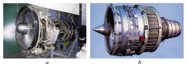
**Figure 3.** Aviation turbojet engine D-36 (*a*); Aviation turbojet engine D-18T (*b*) (Boguslaev & Zhemanyuk, 2000).
