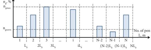
**Figure 2**. Distribution of gas concentrations (carbon dioxide, ammonia, and hydrogen sulphide) ng above the pens:  $n_g - gas$  concentration (carbon dioxide, ammonia, and hydrogen sulphide) above the pens, %;  $n_{gnorm} - limit$  values of gas concentration in the pigsty, %;  $n_{gmax} - maximum$  value value of gas concentration above the pen, %; i - pen number; N - total number of pens;  $L_a - width$  of the pen (provided that the geometric dimensions of all pens are the same), m
