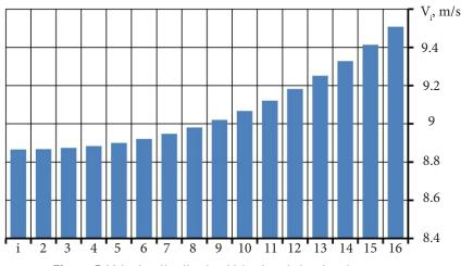
Figure 5. Velocity distribution V, in the air intake pipes
