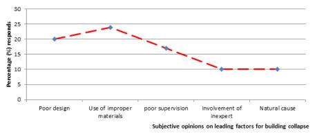
Figure 2. Reported causal factor for building collapse
