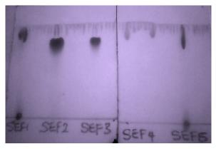
Figure 6: TLC mobility pattern of fractions of *Sapium ellipticum* extract as viewed under ultraviolet lamp at 365 nm
