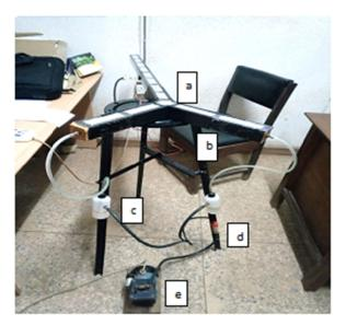
Figure I: Set up showing the connection to the 2way olfactometer: a, 2-way olfactometer; b, metal stand; c, test odour/control container; d, air filter; e, air pump
