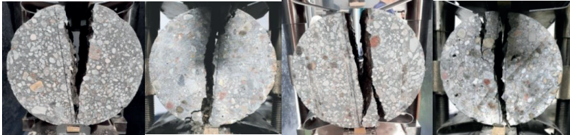
Fig. 7. Examples of the specimens' failure after the tensile splitting test, concrete with natural gravel aggregate (from the left): cylinder 150 \times 300 , C/W = 1.8 ; cylinder 150 \times 150 , C/W = 1.8 ; cylinder 150 \times 300 , C/W = 2.6 and cylinder 150 \times 150 , C/W = 2.6
