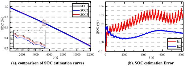
Figure 19: SOC variation curves for three different methods
