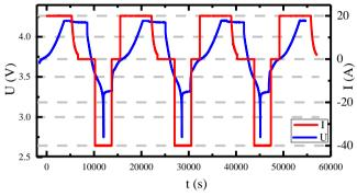
Figure 14: Voltage/Current discharge variation curve
