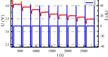
Figure 16: Voltage/Current discharge variation curve
