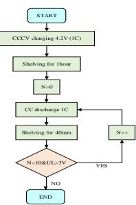
Figure 8: OCV experiment process
