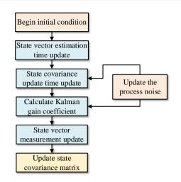
Figure 2: The SOC estimation process using the AEKF algorithm
