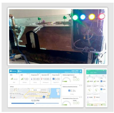
**Figure 5.** Laboratory environment with sensors coupled in a flood scenario and visualization on web and mobile dashboards.
