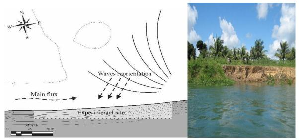
**Figure 3.** Topo/bathymetry showing the wind compass of prevailing winds and reorientation of the wave front, and the thalweg (dashed line) of a concave river bank. **Source:** Rocha *et al.* (2013).
