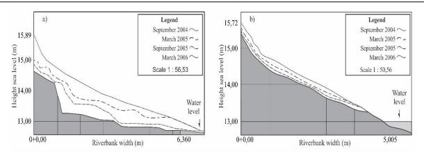
**Figure 7.** Comparison of river bank profiles: left panel untreated river bank; right panel riverbank treated with soil bioengineering techniques. **Source:** Holanda *et al.* (2008).
