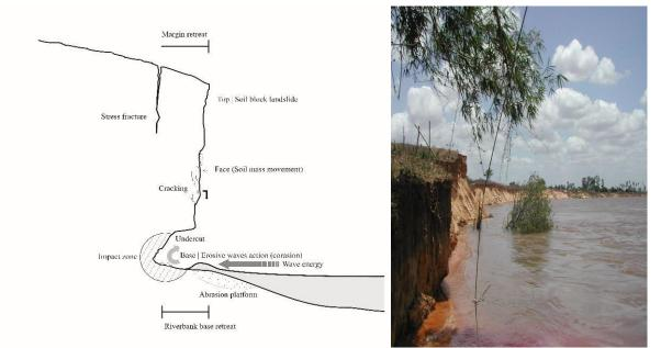
**Figure 4.** Undercutting and failure of river banks along the Lower São Francisco (36°47'28.6" W and 10°13'40.8" S).
