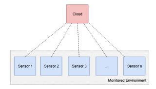
Fig. 1. Cloud Computing-Centred IoT Architecture
