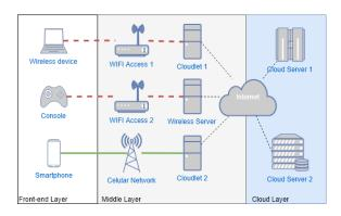
Fig. 4. Mobile Cloud Computing Architecture
