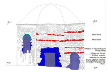
Figure 5: Analysis of the northwest facade. (Drawing: Authors. Red: Ottoman stone rows; green, blue and purple: structures added after the Ottoman times.)
