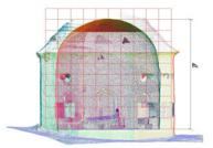
**Figure 15:** The section of the shrine of Idris Baba: the horizontal orthogonal photo based on the point cloud generated by TLS scanner with a modular grid system of the *arşın* unit. (Survey and drawing: Authors, 2019)
