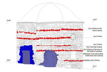
**Figure 4:** Analysis of the west facade. (Drawing: Authors. Red: Ottoman stone rows; blue and purple: structures added after the Ottoman times.)
