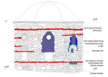
**Figure 10:** Analysis of the south facade. (Drawing: Authors. Red: Ottoman stone rows; green, blue and purple: structures added after the Ottoman times.)
