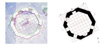
**Figure 13-14:** The plan of the shrine of Idris Baba: the horizontal orthogonal photo based on the point cloud generated by TLS scanner, and the survey drawing based on the point cloud with a modular grid system of the *"arşın"* unit. (Survey and drawing: Authors, 2019)
