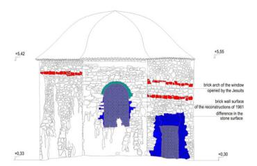
Figure 6: Analysis of the north facade. (Drawing: Authors. Red: Ottoman stone rows; green, blue and purple: structures added after the Ottoman times.)
