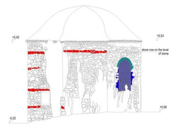
Figure 7: Analysis of the northeast facade. (Drawing: Authors. Red: Ottoman stone rows; green, blue and purple: structures added after the Ottoman times.)
