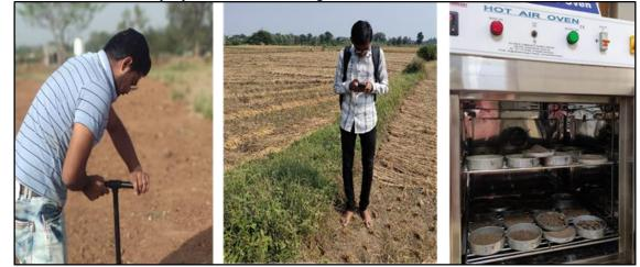
Figure-4: Soil Samples collection in the field and Oven drying of soil samples.
