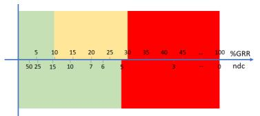
Figure 2. Acceptance/rejection zones according to ndc and %GRR
