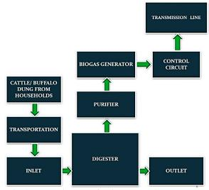
Fig. 2. Block diagram of union based biogas plant.
