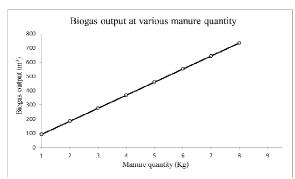
Fig.6. Biogas output for different manure quantities (Per union under the study area)
