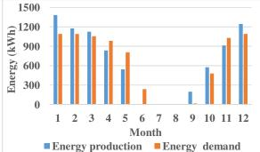
Fig.2. Heating energy demand and energy production for the proposed system
