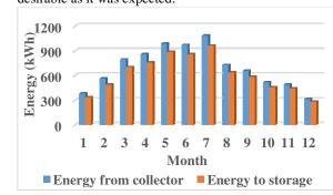
Fig.8. Profile of supplied solar energy from the collector and to the storage tank
