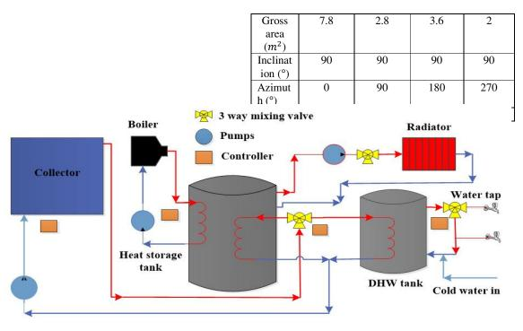
Fig. 1. Space and domestic hot water system for residential application
