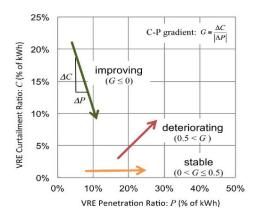
Fig. 2 The concept of the G-indicator [4]
