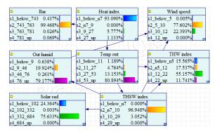
Fig. 5 Conditional probabilities of meteorological variables classes for the first time step
