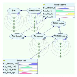
Fig. 10 The dynamic conditional probabilities for wind speed and solar irradiance generated by DBN
