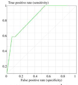
Fig. 8 ROC for class s4 [up 684 W/m<sup>2</sup>] of solar irradiance and AUC=0.6974
