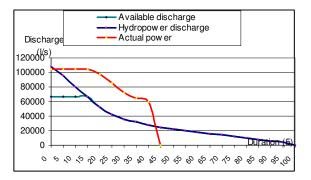
Fig. 8. Flow and Power duration curves
