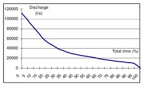
Fig. 6. The Flow duration curve
