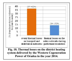
The highest share of (20-25)% heat losses is located on the primary network, while on the distribution pipelines it has values of (14-15)%, compared with 15 % registered by the both, primary and secondary upgraded systems, made from pre-insulated pipelines, (figure 18), [5]
