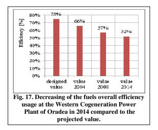
The age of the hot water district network, registered after (35-40) years of running, has caused a large number of failures, consisting of pipe corrosion, main valves locking, demage of the thermal insulation, so that the overall thermal losses of the entire district network reached a share of (40-42) % from the thermal flow delivered by the power plant at its boundary, [5].
