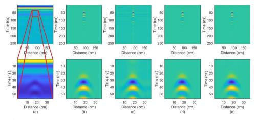
**Figure 4.** First Row: Original Results, Second Row: Zoomed Version: a) raw data, b) reference data clutter suppression results for, c) PCA, d) RPCA, e) TRPCA.
