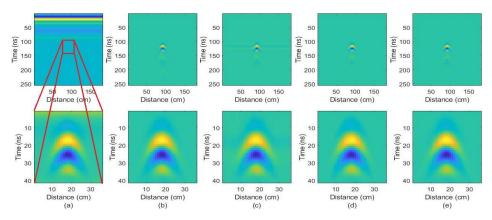
**Figure 5.** First Row: Original Results, Second Row: Zoomed Version: a) raw data, b) reference data clutter suppression results for, c) PCA, d) RPCA, e) TRPCA.
