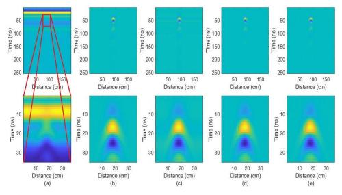
**Figure 6.** First Row: Original Results, Second Row: Zoomed Version: a) raw data, b) reference data clutter suppression results for, c) PCA, d) RPCA, e) TRPCA.
