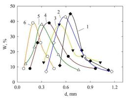
Fig. 4. Particle size distribution of the sorbents:  $TiO_2$  (1) and  $TiO_2$  containing spinel  $LiMn_2O_4$  (2–6). The molar ratio of Ti: Mn was 1:0 (1), 1:0.05 (2), 1:0.1 (3), 1:0.2 (4), 1:0.3 (5) and 1:0.4 (6)
