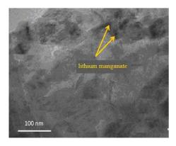
Fig. 3. TEM image of nanocomposite containing HTD and LiMn<sub>2</sub>O<sub>4</sub> (before calcination)
