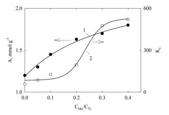
Fig. 7. Dependence of the summary sorption capacity towards Li<sup>+</sup> and Na<sup>+</sup> ions (1) and Li<sup>+</sup>/Na<sup>+</sup> selectivity coefficients (2) on the molar ratio of Mn and Ti ratio in sorbents
