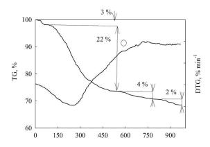
Fig. 1. Data of thermogravimetric analysis of HMD Li-form. The circle indicates the exopeak, which corresponds to the formation of  $LiMn_2O_4$
