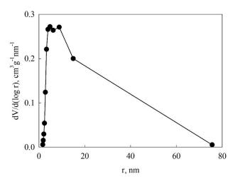
Fig. 6. Differential pore size distribution of LiMn<sub>2</sub>O<sub>4</sub>
