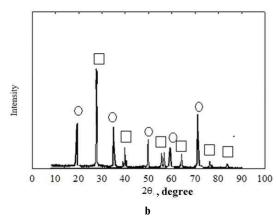
Fig. 2. X-ray diffraction pattern:  $a - LiMn_2O_4$  spinel (white circles) containing  $Mn_2O_3$  traces (black circles), and b - composite containing anatase (squares) and  $LiMn_2O_4$  (circles)
