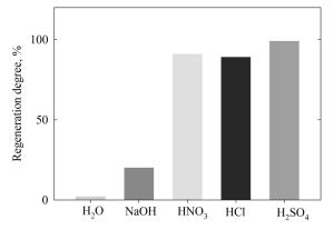
Fig. 8. Regeneration of the sorbent containing LiMn<sub>2</sub>O<sub>4</sub>
