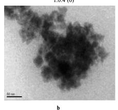
Fig. 5. a - Micrograph of composite granules and b - TEM image of the original spinel nanoparticles incorporated into TiO<sub>2</sub>. The molar ratio of Ti:Mn was 1:1 (a) and 1:0.05 (b)
