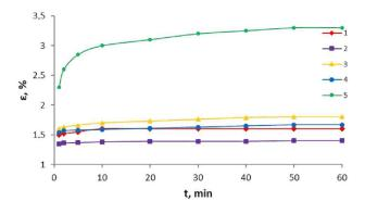
Fig. 9. Creep curves of specimens based on the initial (1, 2) and modified ORH (3, 4, 5) ED-16 epoxy resin, cured by modes I (1, 3, 5) and II (2, 4). Test temperature was 22°C (1, 2, 3, and 4) and 35°C (5)
