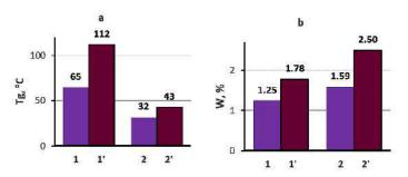
Fig. 3. Glass transition temperature Tg (a) and water absorption W (b) for samples based on the original (1, 1') and modified (2, 2') resins. Specimens were cured by modes I (1, 2) and II (1', 2')
