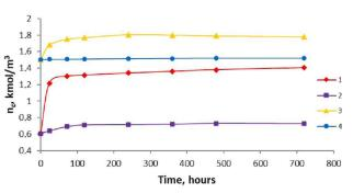
Fig. 7. Dependence of the density of the chemical network  $n_c$  on the holding time  $t_c$  for samples based on the original resin, cured in modes I (1, 2) and II (3, 4): 1 and 3 – exposure in water; 2 and 4 – holding in air
