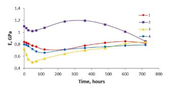
Fig. 8. Dependence of the elastic modulus E on the exposure time  $t_e$  for samples based on the original (1, 2) and modified (3, 4). Specimens were cured by modes I (1, 3) and II (2, 4)
