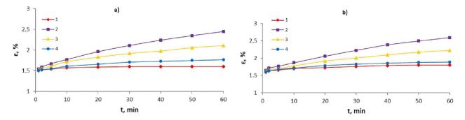
Fig. 10. Creep curves for composites based on the initial (a) and modified (b) resins cured according to mode I. The samples were soaked in water for 0 (1), 24 (2) and 240 (3, 4) hours: 1 and 4 - air tests; 2 and 3 - in water
