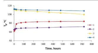
Fig. 6. Dependence of the glass transition temperature  $T_g$  on the exposure time  $t_e$  for samples based on the original resin, cured by modes I (1, 2) and II (3, 4): 1 and 3 – exposure in water; 2 and 4 – exposure in air
