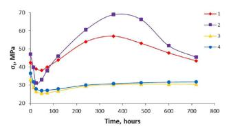
Fig. 4. Tensile strength  $\sigma_t$  vs. exposure time  $t_e$  in water for specimens based on initial (1, 2) and modified (3, 4) resins. Specimens were cured by modes I (1, 3) and II (2, 4)
