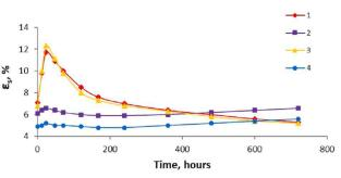
Fig. 5. Dependence of deformation at rupture  $\varepsilon_s$  vs. the exposure time  $t_e$  in water for specimens based on the initial (1, 2) and modified (3, 4) resins. Specimens were cured by modes I (1, 3) and II (2, 4)
