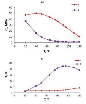
Fig. 2. Tensile strength  $\sigma_t$  (a) and deformation at rupture  $\varepsilon_s$  (b) vs. temperature for epoxide polymers based on initial (1) and modified (2) ORH resins. The specimens were cured by mode II
