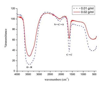
Fig. 6. FT-IR bands of the Cdots samples
