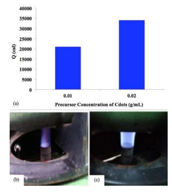
Fig. 9. (a) – Heat performance test; fire texture of biogas from Cdots purification with precursor concentrations of 0.01 g mL<sup>-1</sup> (b) and 0.02 g mL<sup>-1</sup> (c)
