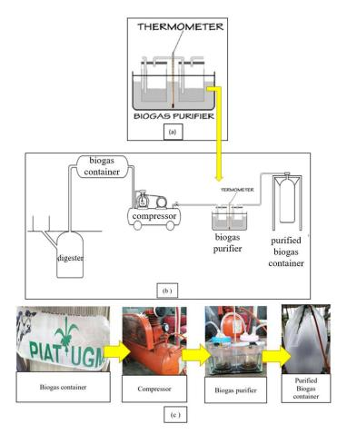
Fig. 1. The biogas purification process: (a) the purifier tube, (b) the scheme of biogas purification and (c) purification procedure
