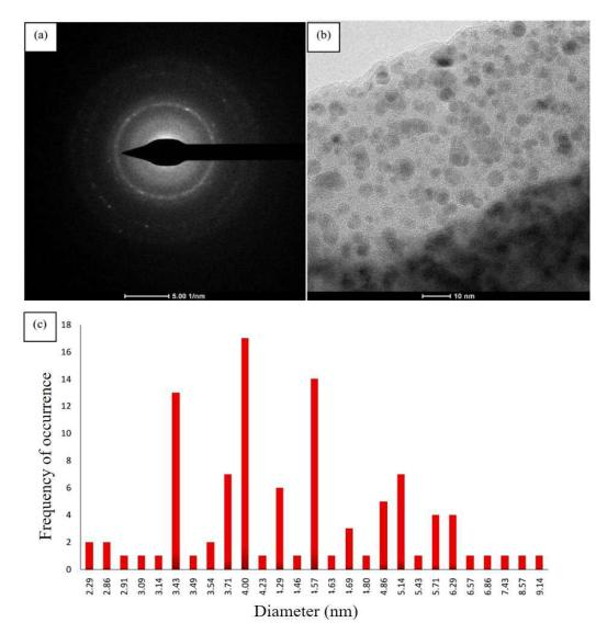
Fig. 7. TEM analysis results: (a) diffraction pattern of Cdots, (b) morphology and (c) diameter distribution of the Cdots
