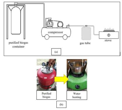
Fig. 2. Heat performance test process: (a) the apparatus for heat performance test and (b) the heat performance test procedure
