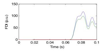
Figure 5: Detection Results of Wavelet Entropy Method for AB Fault.
