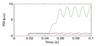
Figure 13: Detection Results of Wavelet Entropy Method for High Resistive BG Fault.
