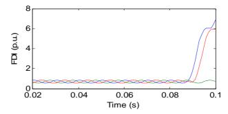
Figure 10: Detection Results of Wavelet Entropy Method for ACG Fault.
