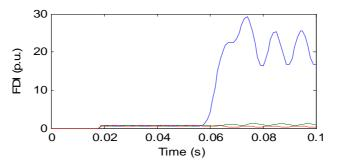
Figure 2: Detection Results of Wavelet Entropy Method for AG Fault.
