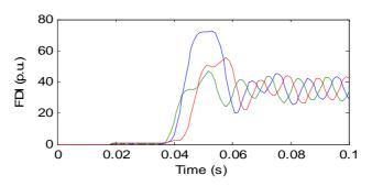
Figure 11: Detection Results of Wavelet Entropy Method for ABCG Fault.
