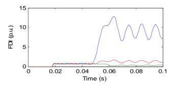
Figure 12: Detection Results of Wavelet Entropy Method for Far-end LG Fault.
