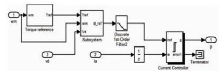
Figure 3: Sub-System Implementation of MPPT control for Wind Power System.
