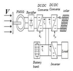
Figure 1: Block Diagram of PV-Wind Hybrid System.
