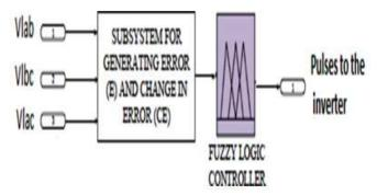
Figure 5: Block Diagram of FLC Voltage Regulated Inverter.
