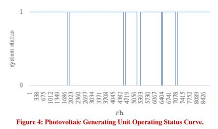
The normal operation-fault-normal operation state sequence of each generating unit obtained in Figure4 is combined with the annual power generation curve obtained in Figure3 to obtain the annual microgrid power generation situation considering the generator unit failure.
