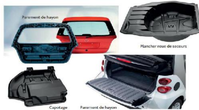
Figure 1: Example of An Automotive Part Made of Composite Materials.
