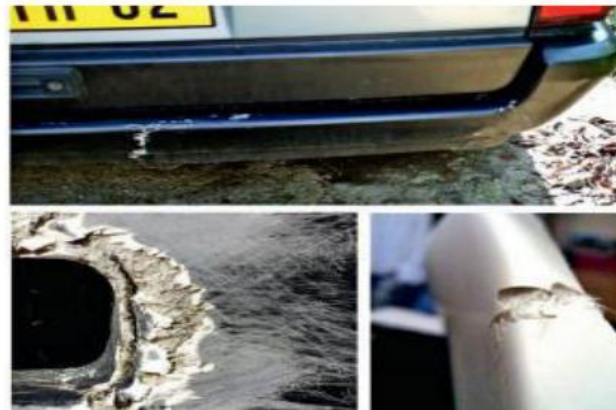
Figure 2: Impacts on the Bumper.
