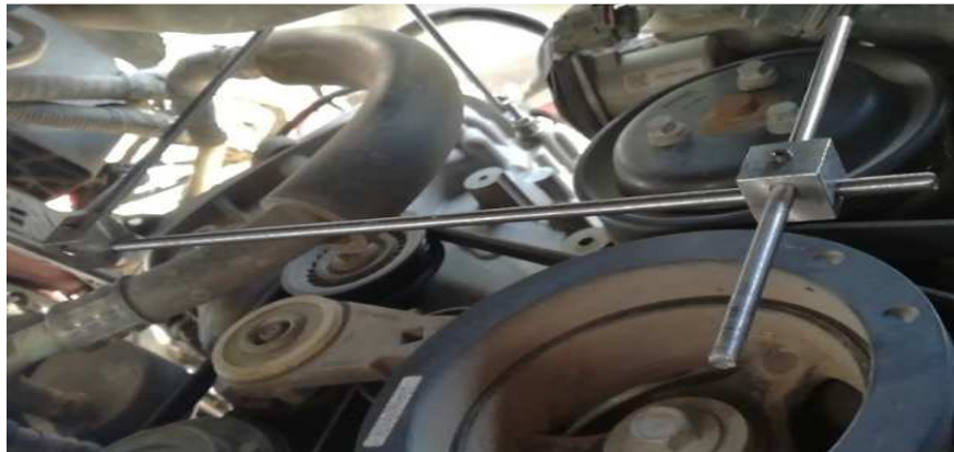
Figure 14: Installing AISI-1050 Carbon Steel Mechanism.
