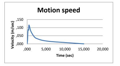
Figure 2.10. Speed growth graph when cylinder retraction
