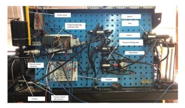
Figure 2.3. Picture of the hydraulic system and component labeling
