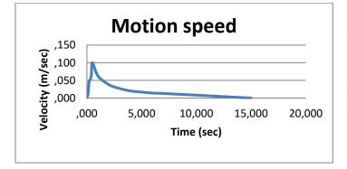
Figure 2.9. Speed growth graph when cylinder extraction
