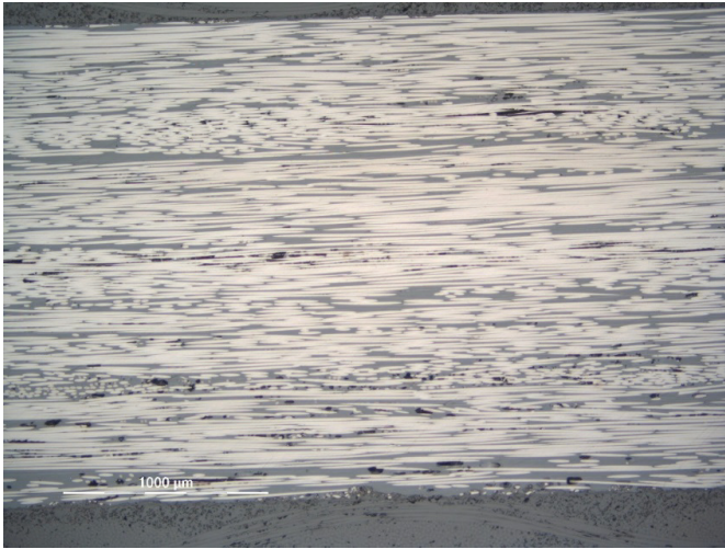
Fig. 15. In-plane waviness of fibres [13].
