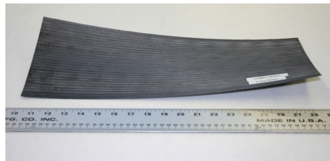
Fig. 14. Distorted flat plate, made from unidirectional layers [12].
