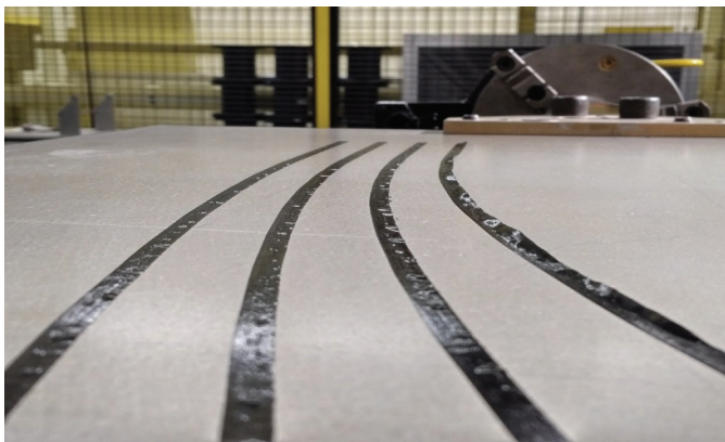
Fig. 10. Fold overs due to fibre steering (in the band with smaller radius).
