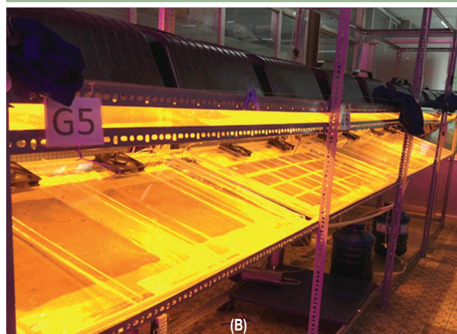
Fig. 6. (A) Diagram of chamber and light source positioning in 2 m 2 system; (B) The 2 m 2 system in use with H. pluvialis on the biofilm.
