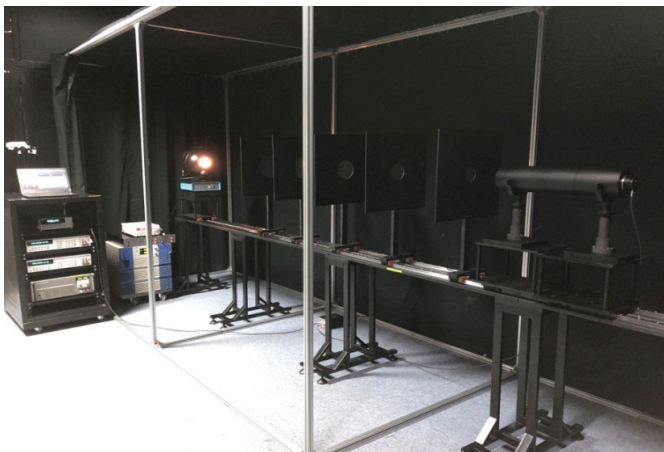
Fig. 2. Photograph of the typical luminance measurement setup.
