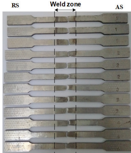
Fig. 5. Tensile specimens and the tensile fracture locations (the dash lines present the tool shoulder).
