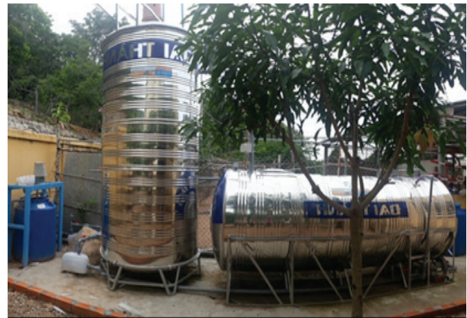
Fig. 1. The pilot scale AnMBR-CSTR model.
