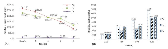
Fig. 7. Effect of electrolysis time on (A) heavy metal concentration and (B) efficiency of removal of heavy metals from COD wastewater.
