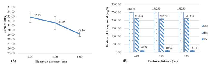
Fig. 6. Effect of the distance between electrodes on (A) the current, (B) the effect of heavy metal removal in COD wastewater treatment.
