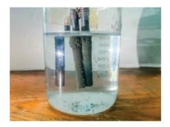
Fig. 11. Wastewater and electrode after treatment process.
