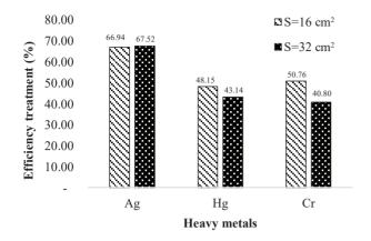
Fig. 10. Comparison of the treatment efficiency of heavy metals between the two electrode areas, 16 and 32  $cm^2$ , for t=8 h.
