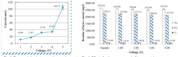
Fig. 2. The correlation between voltage and current. Fig. 3. Effect of voltage on removal of heavy metals.
