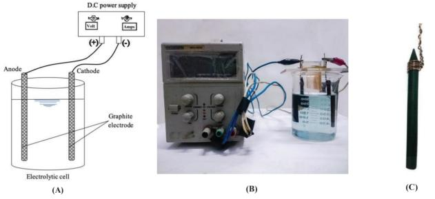
Fig. 1. Electrolytic model of COD wastewater treatment using graphite electrode. (A) drawing, (B) actual model, (C) graphite electrode.
