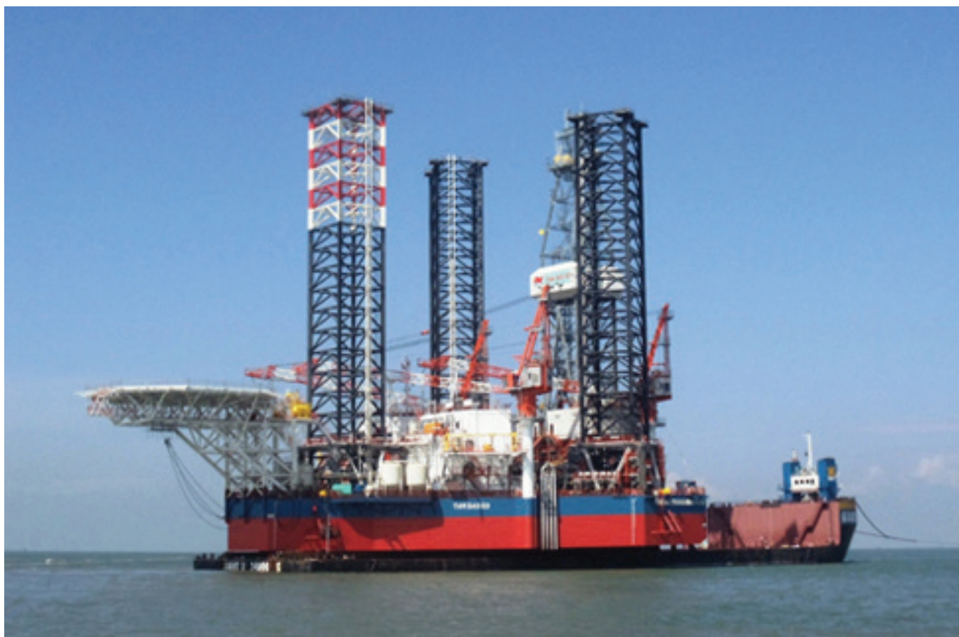
Fig. 1. The 90 m water depth Tam Dao 03 rig marked a breakthrough in the science and technology understanding of the PV Shipyard, and laid a foundation for the design and manufacture of drilling rigs for the industry in Vietnam. Source: pvn.vn.
