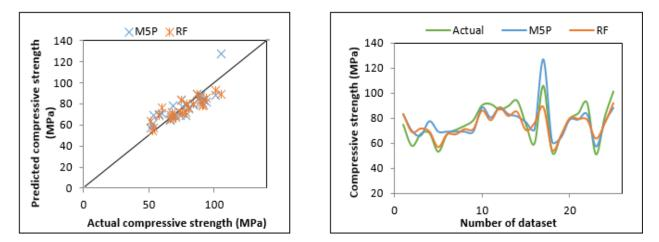
Fig. 5. (a) and (b) Scattered diagram and comparison of actual and predicted values of compressive strength by using M5P model tree and random forest regression in testing dataset
