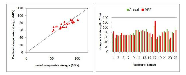
Fig. 3. (a) and (b) Scattered diagram and comparison of actual and predicted values of compressive strength by using M5P model tree in testing dataset
