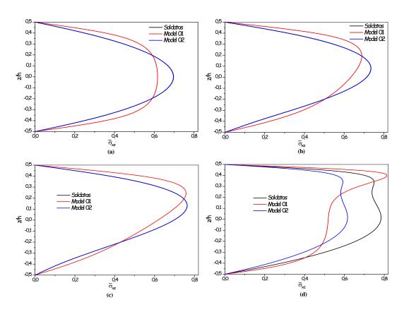
Figure 4: Dimensionless transverse shear stress variation  $\overline{\sigma}_{xz}(0,z)$  through the thickness of the FGM beam under uniform load with (L=2h). (a) P=0, (b) P=0.5, (c) P=1 and (d) P=10.
