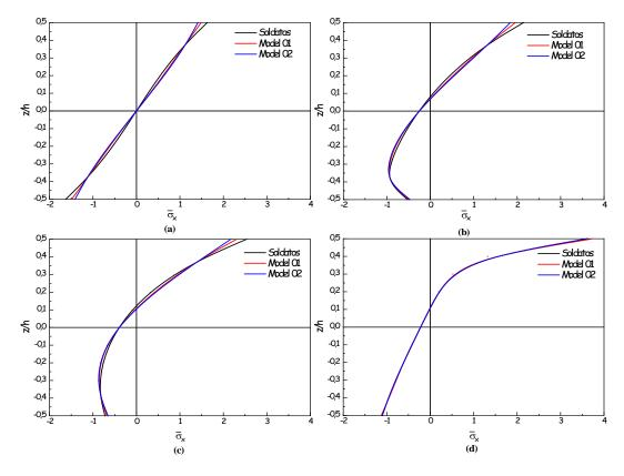
Figure 3: Dimensionless axial stress variation  $\overline{\sigma}_x(L/2,x)$  through the thickness of the FGM beam under uniform load with (L=2h). (a) P=0, (b) P=0.5, (c) P=1 and (d) P=10
