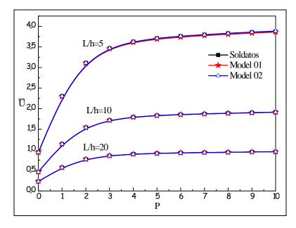
Figure 5: Variation of the non-dimensional axial displacement  $\overline{u}$  as a function of the power law index p for beams FG subjected to a uniform load with different L/h ratio.
