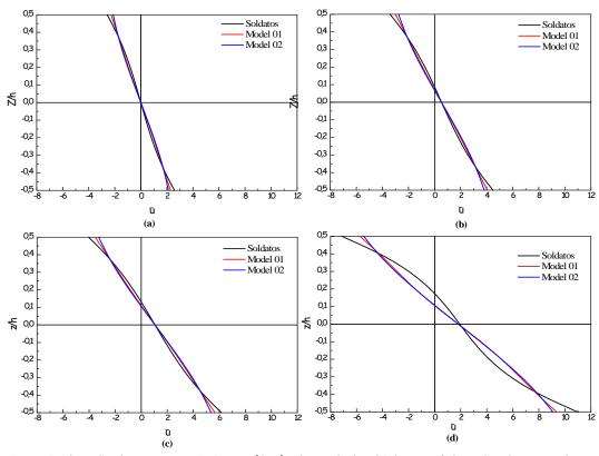
Figure 2: Dimensionless displacement variation  $\overline{u}(0,z)$  through the thickness of the FGM beam under uniform load with (L=2h). (a) P = 0, (b) P = 0.5, (c) P = 1 and (d) P = 10.
