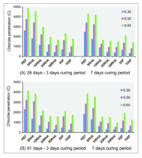
Fig. 4- Chloride penetration results [37]
