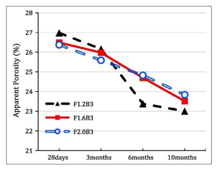
Fig. 2- Effect of Fly ash on Apparent porosity [32]
