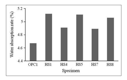
Fig. 1- Water absorption rate of specimens [26]
