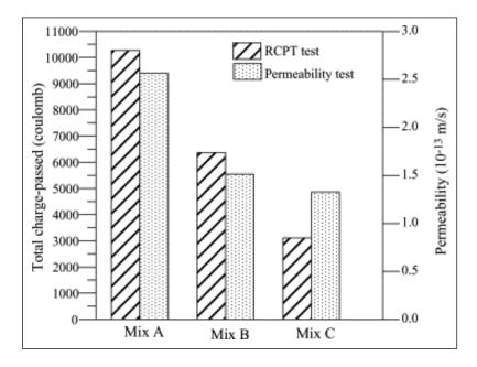
Fig. 5- Total charged passed for chloride penetration [46].
