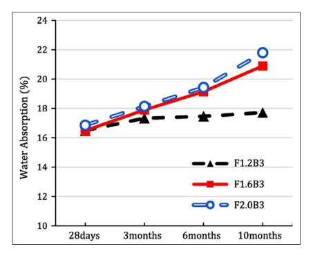
Fig. 3- Effect of Fly ash on Water absorption [32]
