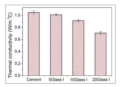
Fig. 6- Thermal conductivity of pastes [73]
