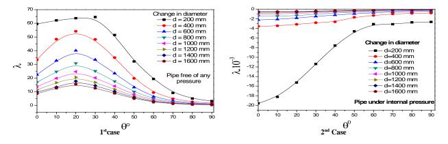
Fig. 2–Influence of the variation of the diameter of the pipe-buckling coefficient depending on  $\theta$
