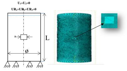
$\label{eq:U1} U_1=U_2=U_3=UR_1=UR_2=UR_3=0$  Fig. 6-Representation of boundary conditions and the pipeline with a square mesh notch
