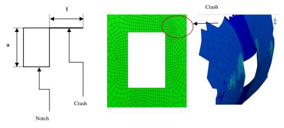
Fig. 10-The pattern and mesh at the notch and the longitudinal crack
