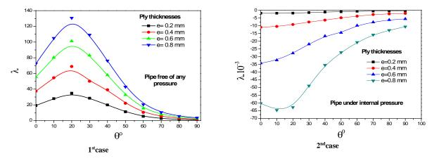
Fig. 3–Influence of the variation of the thicknesses of the pipe on the buckling coefficient in function of  $\theta^{\bullet}$
