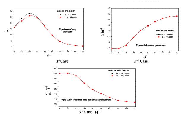
Fig. 9–Influence of size of the notch on the buckling factor as a function of  $\theta^{\bullet}$ , for a pipe provided with dual, square notches
