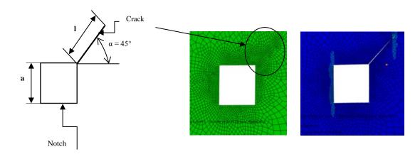
Fig. 15-the pattern and mesh at the cut and the crack inclined at  $\alpha = 45^{\circ}$
