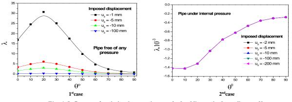
Fig. 4–Influence of variation in restraints on the buckling ratio depending on  $\theta^{\bullet}$
