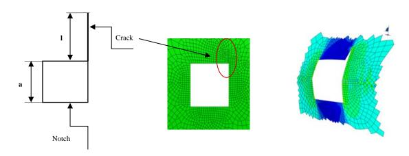
Fig. 13–The pattern and mesh at the notch and the crack inclined at  $\alpha = 90^{\circ}$
