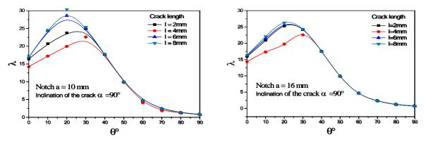
Fig. 14–Buckling parameter variation depending on the orientation of the plies (transverse crack)
