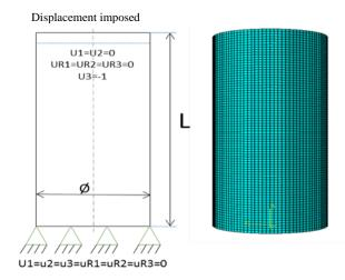
Fig.1-Representation of the boundary conditions and mesh pipeline unnotched
