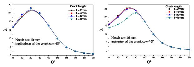
Fig. 16–Buckling parameter variation depending on the orientation of the plies (Crack inclined at 45<sup>•</sup>)
