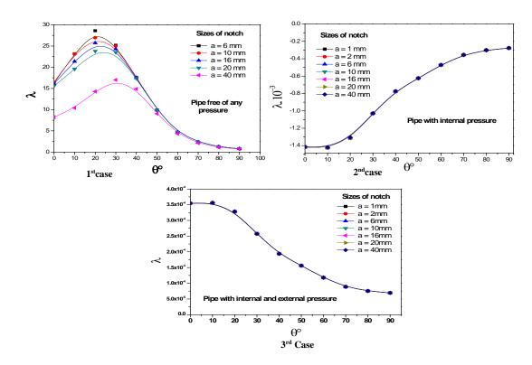
Fig. 7–Influence of size of the notch on the buckling factor as a function of  $\theta^{\bullet}$ , for a pipe provided with a single notch
