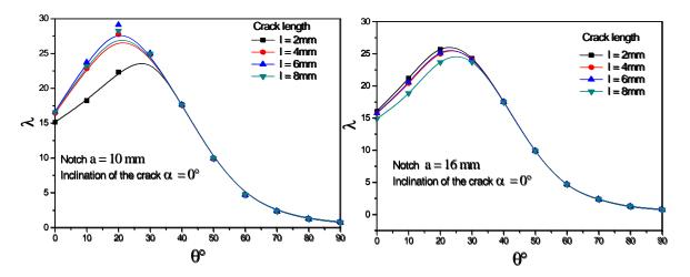
Fig. 11–Buckling parameter variation depending on the direction of the folds for a longitudinal crack
