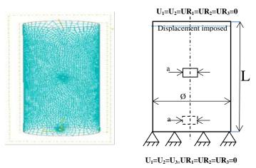
Fig. 8-Representation of the boundary conditions and pipe mesh with two square notch
